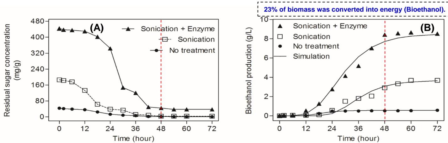
**Figure.** Residual sugar concentration (A), Cumulative bioethanol production (B), during SHF of microalgae *C. mexicana* for 3 days.
