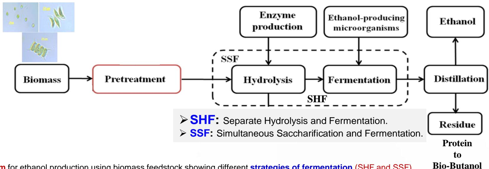
**Flow diagram** for ethanol production using biomass feedstock showing different **strategies of fermentation (SHF and SSF)**.
