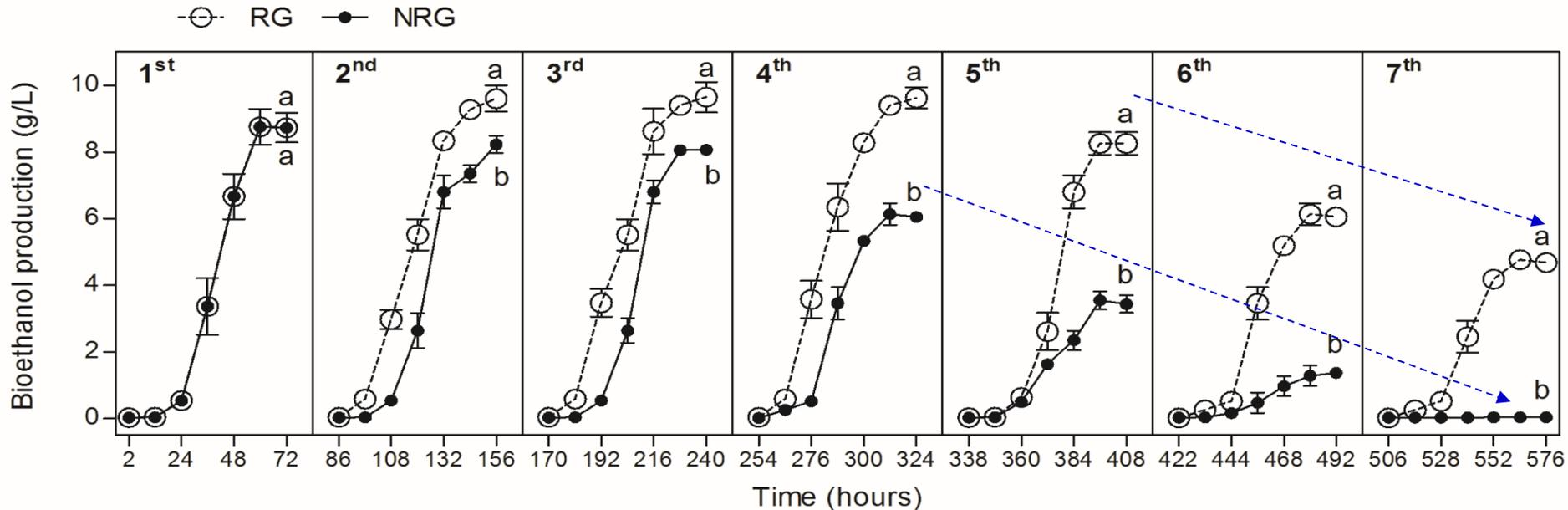
**Figure.** Cumulative bioethanol production from *Chlamydomonas mexicana* through **7-cycles** of repeated fermentation using **immobilized** yeast cells. **RG**: regenerated; **NRG**: non-regenerated beads
