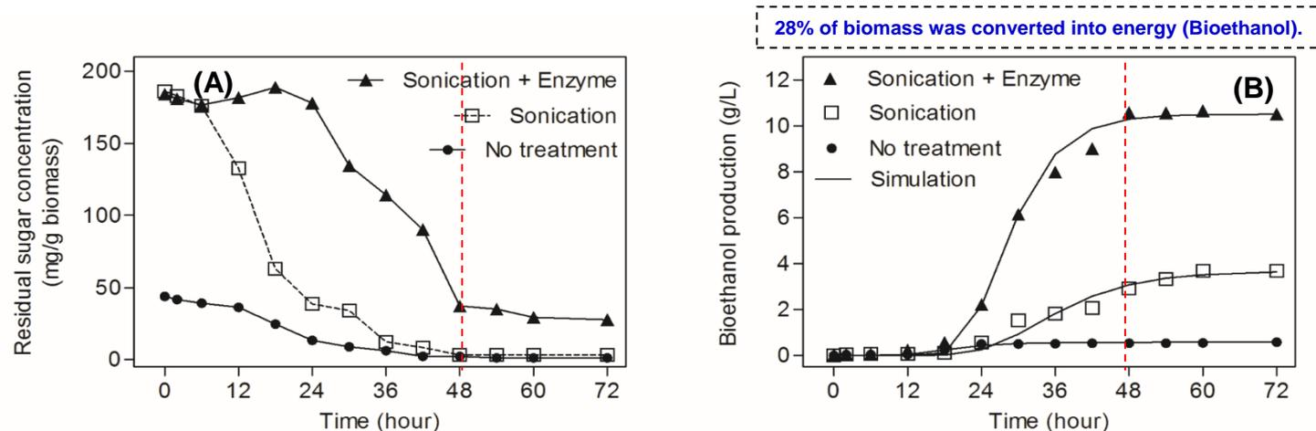
**Figure.** Residual sugar concentration (A), Cumulative bioethanol production (B), during SSF of microalgae *C. mexicana* for 3 days.
